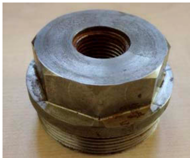
Figure 16-1 1/2" female NPT-2" male NPT. Stainless steel.
