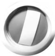
Figure 14-7 Sensor with Carbon/polymer Strip
